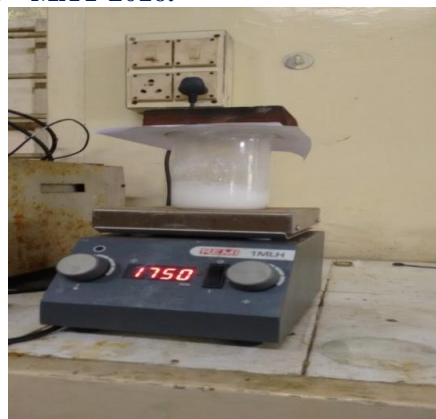
Fig 2.7. Shows hydrolysis + stirring and addition of B 4 C + stirring respectively
