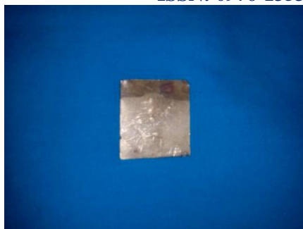
Fig 2.9 Nickel titanium diboride coated on mild steel sample
