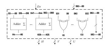
Fig 3 64-bit DMC encoder structure using multi bit adders and XOR gates
