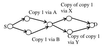
Fig 6: The second copy of RREQ via B is concealed at intermediate node I. Although two copies of the first copy (via A) still reach the destination D. Both are replied to by D even though both carry the same first hop. The reverse paths will combine at I and then divided again. But they will stay link disjoint.
