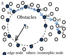
Fig.2.Edge structure without routing void
