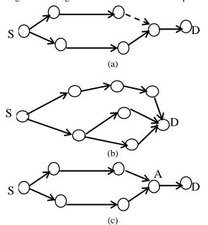
Fig 5: Numerous network configurations explanation various protocol features. (a) Suppose, the second copy of RREQ is transmit over the dotted link. AODV ignore it. But AOMDV forms a reverse path throughout the previous hop. Either protocol does not forward the second copy. (b) Three
