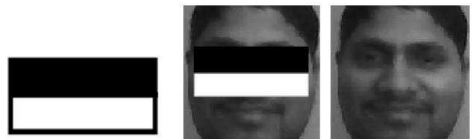
Fig 3: Haar Feature that looks similar to the eye region which is darker than the upper cheeks is applied onto a face.
