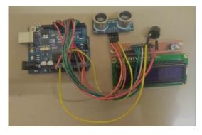
Fig 1(b) Ultrasonic Waist Belt Sensor system
