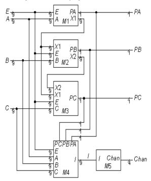
Figure 3 C432 Combinational Circuits
