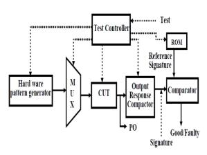
Figure 1 Block diagram of BIST
