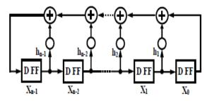
Figure 2 Standard LFSR circuit
