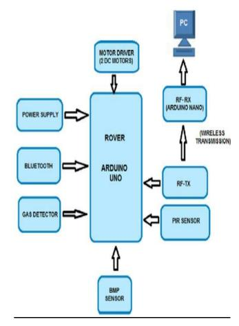
Receiver) in the Transceiver interfaced to the Control Unit (Arduino) on the robot is for sensing the signals transmitted by the RF- Tx (Radio Frequency Transmitter) in the remote. The data received by the RF-Rx is conveyed to the control unit which moves the robot as desired.
