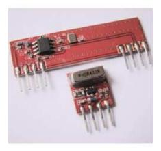
The main application of RF module is an embedded system to communicate with another device wirelessly. This communication may he accomplished through radio frequency communication. For various applications the medium of choice is radio frequency since it does not need line of sight.
