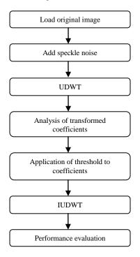
The figure 1 shows the functional procedure of despeckling using UDWT. Here original SAR image is considered and speckle noise is added with different noise variance level from 0.01 to 0.3. In SAR image, Wavelet transform is considered and their Co-efficients are predictable for the transformed SAR image. To reconstruct the transformed image IUDWT is applied and the performance metrics are obtained.
