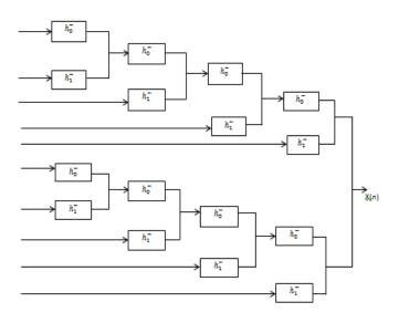
Fig 3: The Inverse dual tree discrete CWT (IDTDCWT) Synthesis (modulation) FB.
