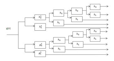
Fig 2: The dual tree discrete CWT (DT-DCWT) Analysis (demodulation) FB.
