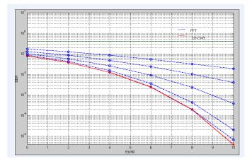
Figure 5: BER performance of FFT-OFDM and DTCWT -OFDM
