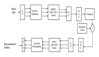
Fig 4: Functional block diagram of OFDM based on DT-CWT
