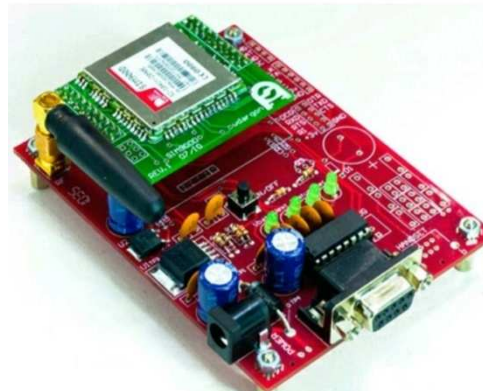
Figure 2. GSM Kit Features
