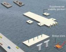
Step 4: Join supplemental pontoons to longitudinal pontoons at staging area. Begin installation of columns on cross pontoon.
