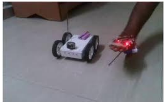
Fig 1 Accelerometer controlled robot vehicle
