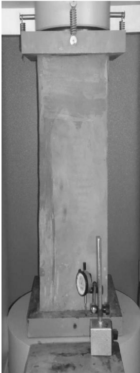
RC Column & Column strengthened by steel angle and strips
