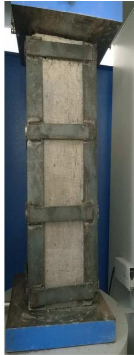
RC Column & Column strengthened by steel angle and strips
