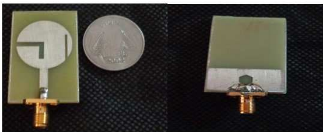
Fig. 6. Top view and Bottom view of the fabricated antenna
