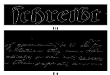
Fig. 2. (a) and (b) Detecting Edge of images using Canny Edge Detection Method
