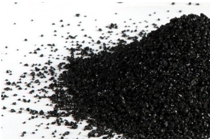
Mineral admixture used (copper slag)
