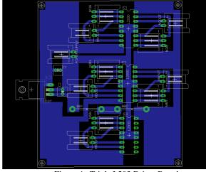
Figure 4 : Triple L293 Driver Board
