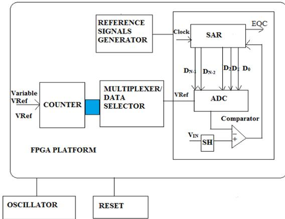
Fig.2 Split SAR ADC- Functional Block Diagram
