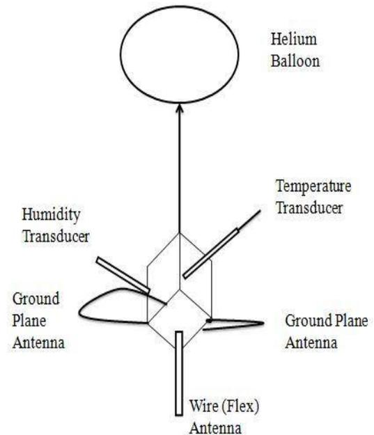
Fig. Radiosonde Measuring Ozone Concentration
