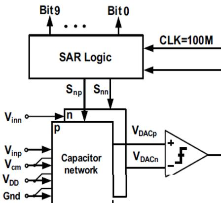
Fig.1 Block Diagram of ADC Architecture
