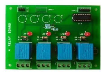
Fig 4. Four Relay Board
