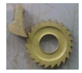
Figure 3: Fabricated Ratchet and Pawl Mechanism
