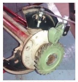
Figure 4: Anti Roll Back Mechanism
