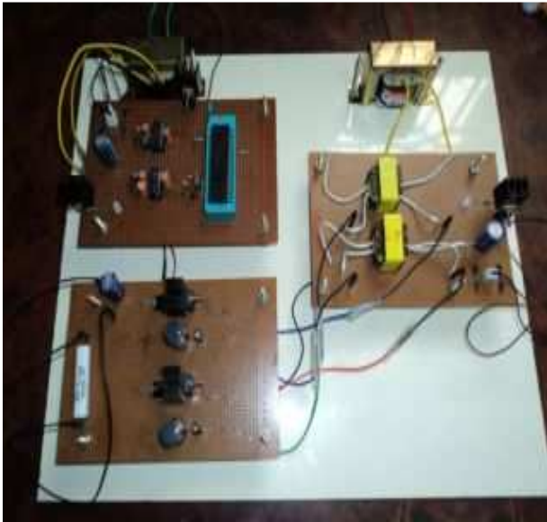
Fig.12 Proposed converter-Experiment prototype
