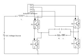
Fig.1. Basic current fed inverter with parallel resonant load.
