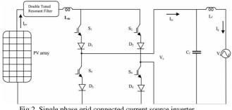
Fig.2. Single phase grid connected current source inverter.
