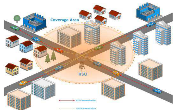
Figure 1. Communication architecture of VANET.
