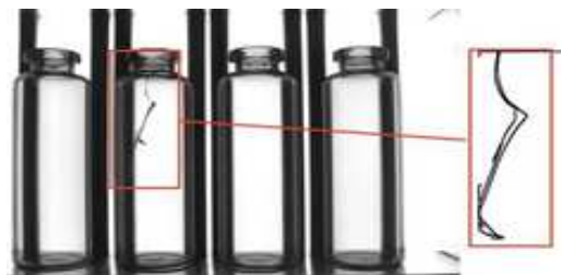
Figure 1.3. Crack defect detection drawing of tube-type bottle body.
