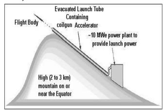
Constructing the EM-Launch station along the mountain slides has lot of advantages. By constructing the launcher at an inclined angle of 25 degrees [3] enables us to eliminate the booster rockets from guiding work. In addition to these things, the mountain will be a good absorber of vibration and sound, which were produced during the launching.
