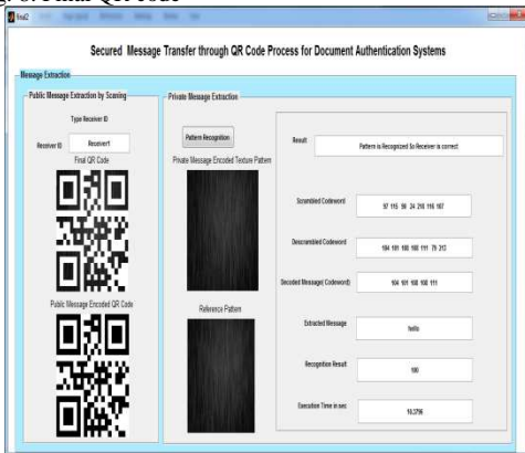
Fig.9. Scanning the public message for performing extraction process. And, the private message is also extracted using decoding process
