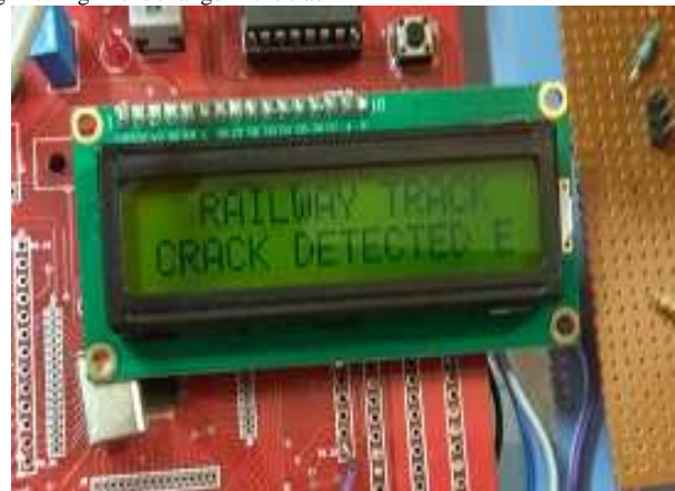
Fig 12. Crack identified in the track
