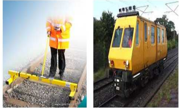
Fig 1. Traditional track inspecting vehicles
