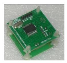
Fig.2 RFID Reader 125 kHz
