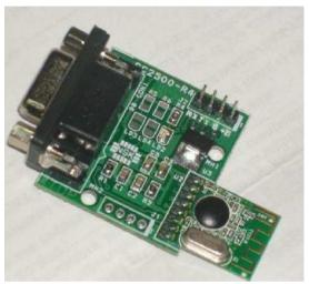
Fig 3. Zigbee Transceiver
