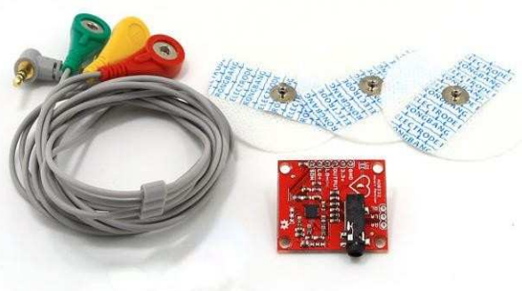
Fig 5: AD8232 ECG Sensor with electrode and connector cable
