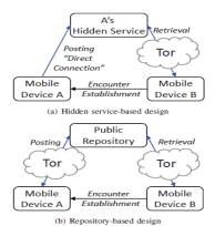
Fig. 1. Two specific designs. Fig. (a) illustrates the first design using Tor hidden services as encounter storage place. Fig. (b) illustrates the second design where users store encounter information on a public replica and gain anonymity to their access using a normal Tor operation.
