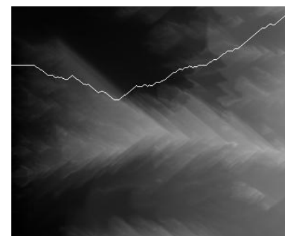
Fig. 10 Energy Map With Horizontal Seam
