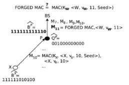
Fig 4: Example of MAC forging during aggregation phase
