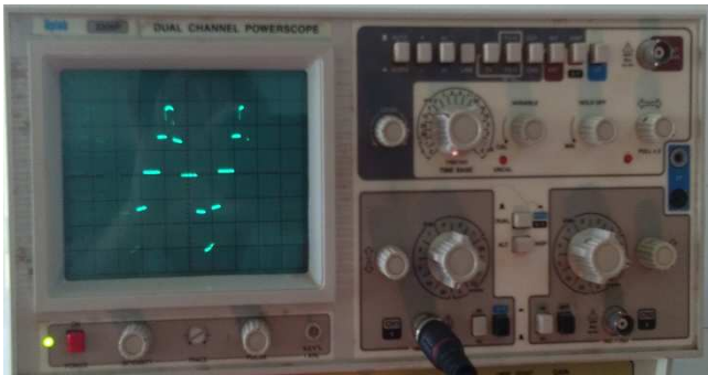
Fig.6.3 Experimental waveform during normal operation of inverter.
