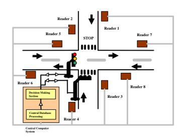
The data thus obtained is then sent to the CCS through wired or wireless channels based on the convenience at the place. The central database processing data. Based on the processed results the DMS controls the traffic lights.
