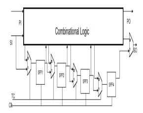
Figure 1.1: Scan chain DfT structure
