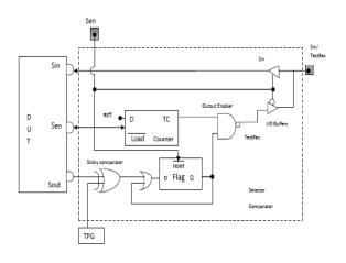
Fig 2 Proposed secure comparator Using Test Pattern Generator
