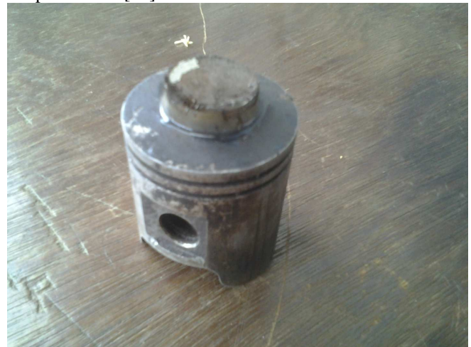
Fig 1: Piston with magnet in top face
