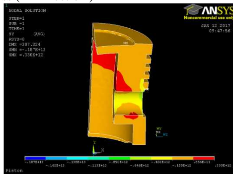
i) Aluminum Alloy Stress ( Y Direction )
